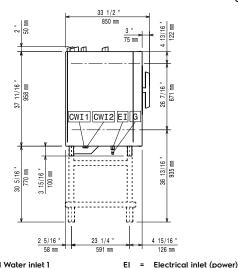
CWII Cold Water inlet 1 CWI2 Cold Water Inlet 2 D
